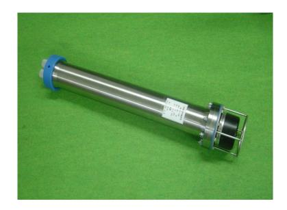
This 11000m transponder is specially developed for operations in the deepest ocean of the world. Underwater vehicles attaching this transponder can be located by acoustic positioning system, and the power on/off switch can be controlled by acoustic command / ranging deck unit.
